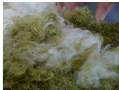
Figure 12 mixing cotton and vetiver fibers of 50:50 ratio
