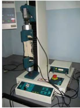
Figure 28 strength testing of fabric per length unit
